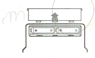
Insert two AA batteries, UM-3 or equivalent making sure to align  $^{\prime\prime}+^{\prime\prime}$  and  $^{\prime\prime}-^{\prime\prime}$  as shown.
